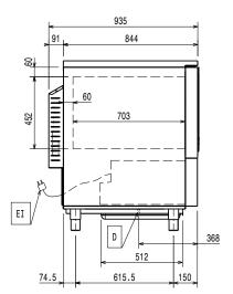
Drain Electrical inlet (power)
